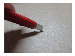
Take your second matte knife and round off the point of the knife by dragging it across a cement floor or sidewalk area. Drag it as if you are trying to cut the sidewalk. This will round off and dull the tip of the blade which is usually the reason we miss cut into the back surface. The blade should look like this tip when you're done.
