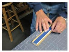
A "sanding bar" is very handy in building. It's a tool that you'll use over and over. It's nothing more than a flat piece of wood wrapped with sandpaper. The length of wood you'll use for this must be flat and smooth. The bar I use was made from a 9" length of furring strip wood that is about 2-1/2" wide and 3/4" thick.
