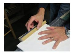
Holding the sanding bar at a 45 degree angle, sand the edge back and forth to create a 45 degree angle on that surface. You can check your progress periodically by testing the movement of the control surface and then return to sanding if more movement is required. This bevel will allow the control surface to now move in both directions.
