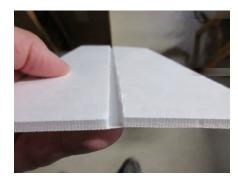
where you cut along the edge of the foam to remove the paper top surface and underlying foam leaving a paper ledge on the bottom surface.
