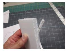
If cut properly, you should be able to pull away the center section of foam creating a channel. This technique is used to create right angle folds in the foam.
