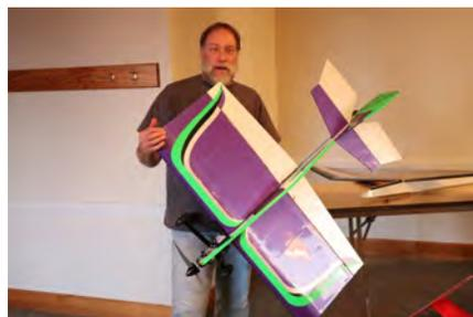
**Dave Kearn** brought his newly refurbished Wild Hots. It features a 10.5" wingspan, E-Flite 32-770kv motor, Hobby Wing 80 amp ESC, and a 4S-3300 mAh battery pack. Flying weight about 4.5 to 5 lbs.
