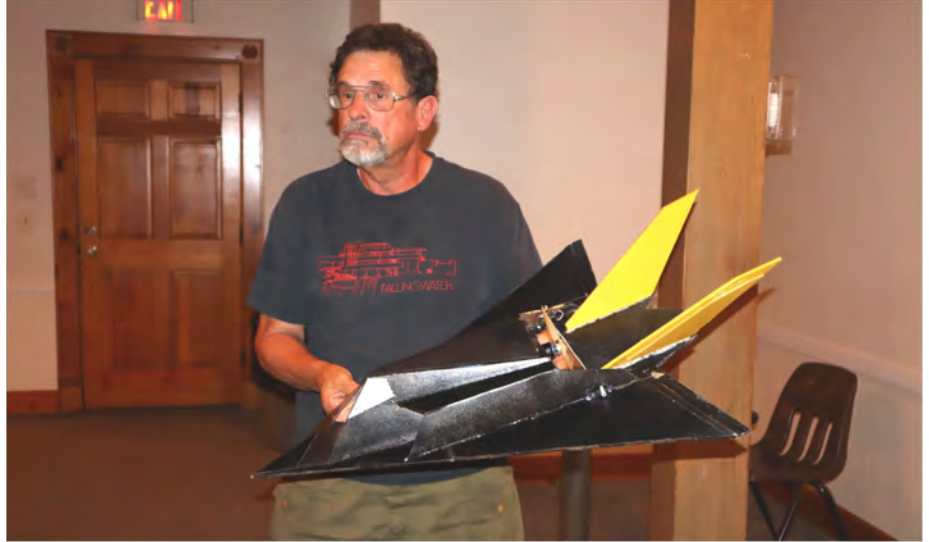
Ed Malec presented his entry to the Builder's Challenge contest, a RC Foam Fighters F-117 made of foamboard and modified tail structure for added strength. The craft uses an Assassin motor, prop, and two servos.
