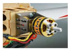
called ESC's (Electronic Speed Controllers) that allow us to flow the power of a LiPo battery to the motor in a graduated way, through a receiver and directed by signals from a transmitter. How cool is that! In fact, electric motors have advanced so much that they can now power ex-
